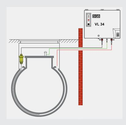
For single-walled tanks with a leak protection lining and other containments with a suction line for the leak detector to the low point of the interstitial space. Not explosion-proof design!
