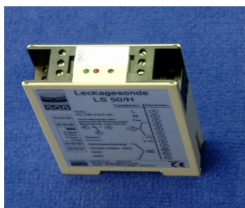
LS 50 leak indicating unit A
