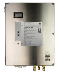
Unique technology bundled in a high-quality stainless-steel housing (IP 54). The vacuum leak detector VLXE – the E stands for full electronic equipment – is specially developed to monitor explosive mixtures in double-walled tanks. For this purpose, the components of the leak detector are partially designed explosion-proof.
