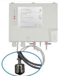
The pressure leak detector DL..8S and the vacuum leak detector VLXE..M8S combine the tried and tested monitoring of double-walled tanks with the monitoring of dome shafts, pump sumps, etc. For this purpose, up to 8 Ex probes (8S) are connected to the leak detector - one per dome shaft. The float switches are explosion-proof and therefore suitable for installation in Zone 1. They react to an increase in liquid in the dome shaft.
