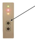
Press the "mute" button once, the audible signal switches off, the respective LED (red for channel 1, yellow for channel 2, and flashing red and yellow for channel 3) lights up.
