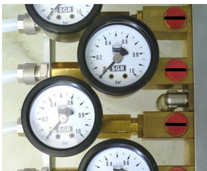
Manifold tank "Measure" with opened valves
