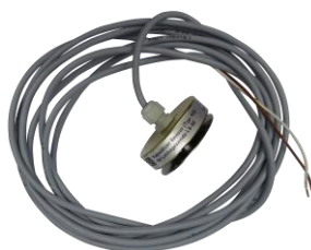
Capacitive sensor KS: 5 m cable, self-supporting Indication level \leq 5 cm Density medium > 0,8 g/cm 3 Temperature -20 ... +70 °C Article no. 105 560
