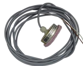
Capacitive sensor with Fleece KVS: 5 m cable, self-supporting Indication level = Amount of liquid to drench fleece Temperature -20 ... +70 °C Article no. 105 565
