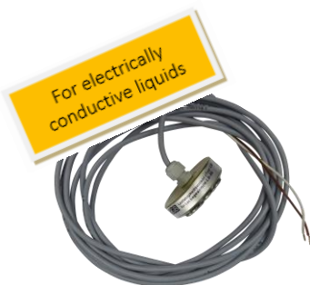
Conductivity sensor LS: 5 m cable, self-supporting Indication level \leq 5 cm Density medium > 0,8 g/cm 3 Temperature -20 ... +70 °C Article no. 105 550
