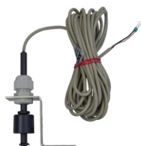
Floating switch FS: PVC, 5 m cable, holder Indication level \leq 3 cm Density medium > 0,8 g/cm 3 Temperature -20 ... +60 °C Article no. 105 531
