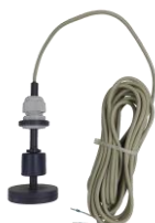
Floating switch FS: PVC, 5 m cable, self-supporting Indication level \leq 3 cm Density medium > 0,8 g/cm 3 Temperature -20 ... +60 °C Article no. 105 535
