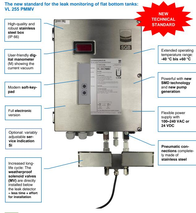
A Class 1 leak detection system according to EN 13160: Every leak – no matter in which of the bottoms – is indicated by an acoustical and optical alarm <u>before</u> the stored product can escape into the environment. The VL 255 PMMV thus fulfills the highest safety requirements in environmental and water protection according to European standards!
